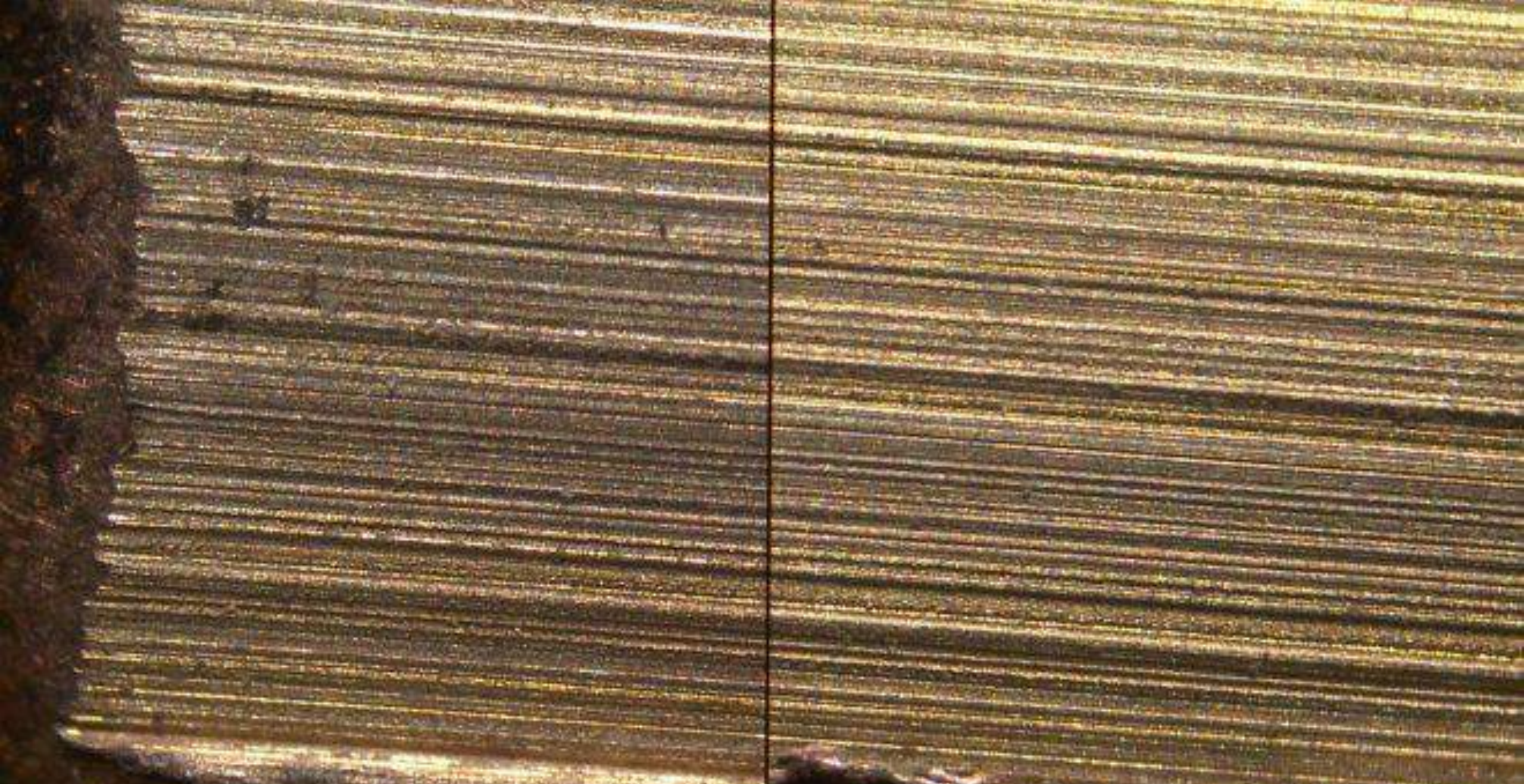
RIFLING (GROOVE) COMPARISON
